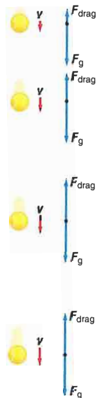
Figure 12 The drag force on an object increases as its velocity increases. When the drag force equals the gravitational force, the object is in equilibrium so it no longer accelerates.
