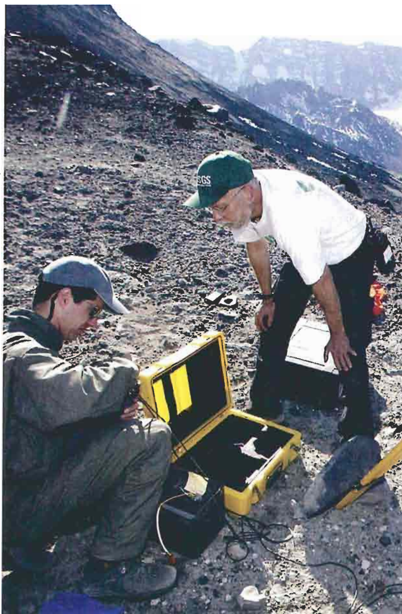
Figure 14 This scientist is setting up a highly accurate GPS receiver in order to record and analyze the movements of continental plates.
