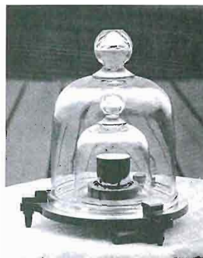
Figure 7 The International Prototype Kilogram, the standard for the mass of a kilogram, is a mixture of platinum and iridium. It is kept in a vacuum so it does not lose mass. Scientists are working to redefine the standard for a kilogram, using a perfect sphere made of silicon.
